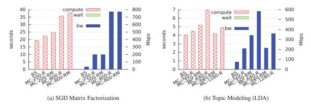
Figure 6: Overhead of communication management: average per-iteration time and bandwidth consumption
