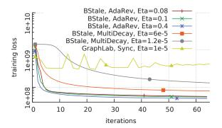
Figure 3: Compare Bösen's SGD MF w/ and w/o adaptive revision with GraphLab SGD MF. Eta denotes the initial step size. Multiplicative decay (MultiDecay) used its optimal initial step size.
