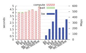
(b) average per-iteration time and bandwidth consumption
