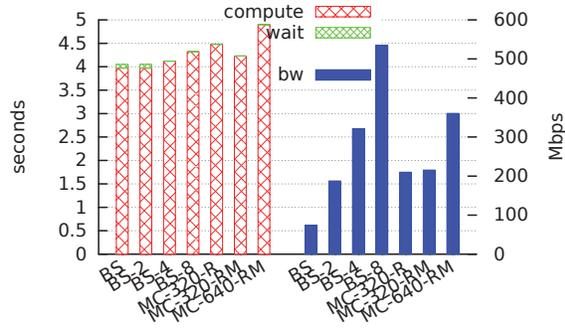
(b) average per-iteration time and bandwidth consumption
